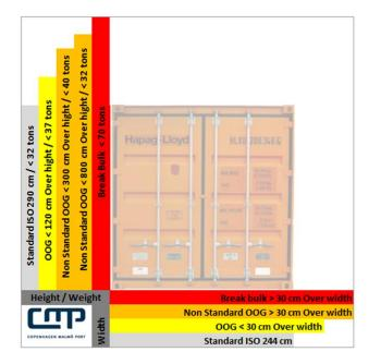
Container dimension: OOG, Nonstandard and Break bulk- containers
