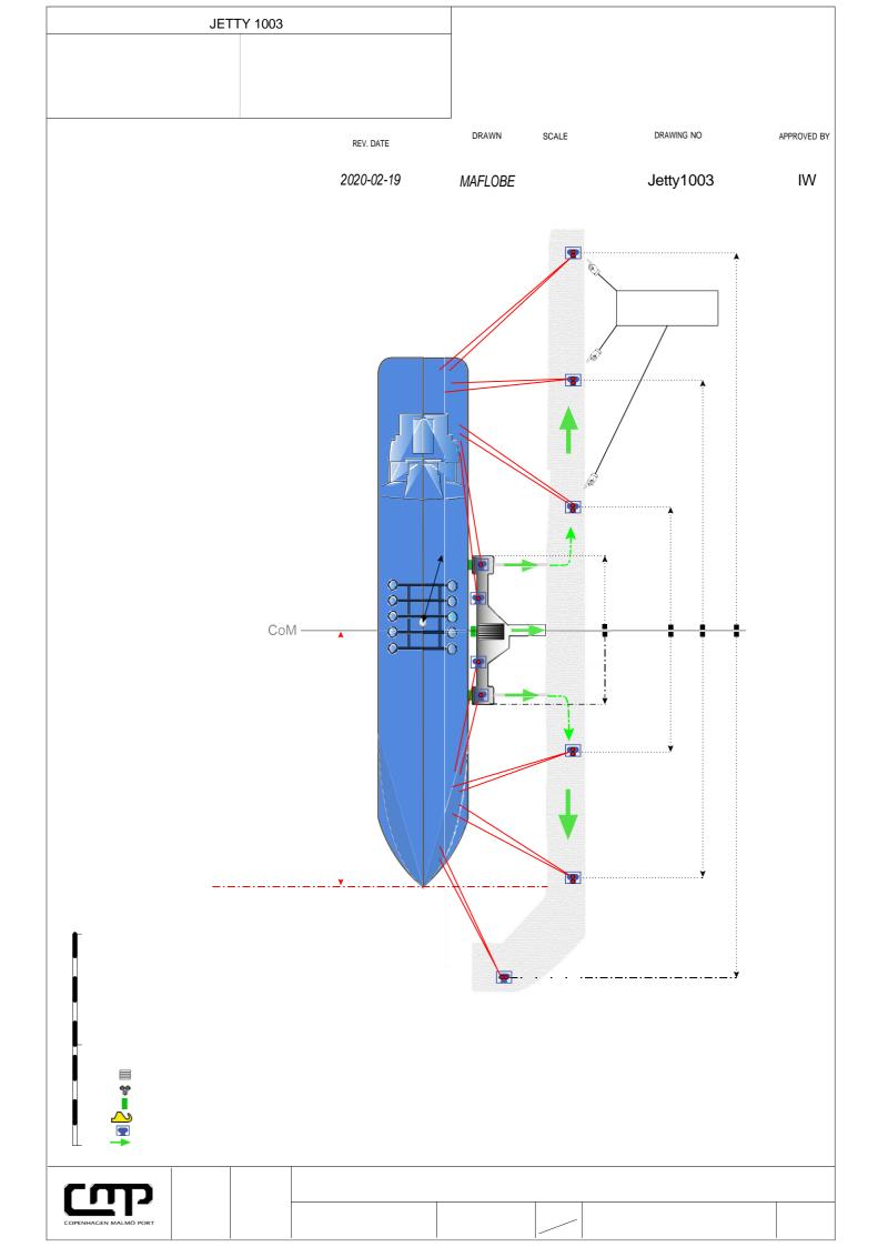
**JETTY 1003** 12,5 m MAX/MIN MANIFOLD HEIGHT MAX DRAUGHT (MW): 250 m ABOVE WATERLINE (MW): N/A MAX LOA: 45 m QUAY DECK HEIGHT (MW): 2,5 m MAX BREADTH: 1,0 m MAX BCM: 120 m UKC: 38 m MAX DISPLACEMENT: N/A MIN PARALLELL BODY: N/A MAX SPEED: N/A MIN FREEBOARD (MW):
