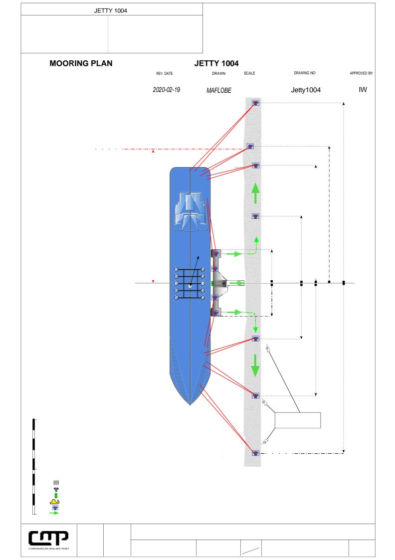
**JETTY 1004** 12,5 m MAX/MIN MANIFOLD HEIGHT MAX DRAUGHT (MW): 250 m ABOVE WATERLINE (MW): N/A MAX LOA: 45 m QUAY DECK HEIGHT (MW): 2,5 m MAX BREADTH: 1,0 m MAX SCM: 140 m UKC: 38 m MAX DISPLACEMENT: N/A MIN PARALLELL BODY: MIN FREEBOARD (MW): N/A MAX SPEED: N/A
